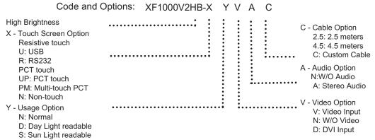
Example: XF1000V2HB-UPSVA2.5 10.4" 600nits backlight with PCAP touch, Sunlight readable, Video, Audio with 2.5m all-in-one cable.
